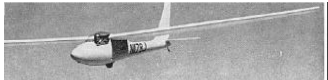
Laister LP-46 – Owner: Orange County Soaring Association. The LP-46 is the prototype for the highly successful LP-49, made by Laister Products in El Monte, CA. Standard Class. 475 lbs empty. 36:1 at 50 mph.
