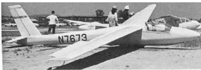
Schweitzer 1-34 – Pilots: Jay Dement, Dan Dickinson, Terry Little, Frank Renek. First one flew in April 1969. 550 lbs. empty, 34:1 @ 55
