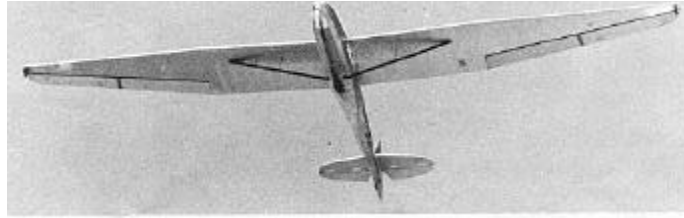
LK-10A (TG-4A) - Owners: Wayne Smith & Allan Krosner, Originally designed in 1942 by Jack Laister. Produced in quantity for the military, this glider was made in 1944. The present owners spent four years rebuilding it. 475 lbs. empty. 22:1 g/r.
