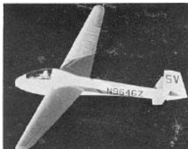
LM-1 – Owner: William C. Meyer. Designed and built in Southern California by Al Leffler, Walt MacFarlane & Bill Meyer. The LM-1 first flew in 1963. It features a two-wheel retractable landing gear. Wings are from an early LK-10 and span 50 feet. 693 lbs. empty 30:1 g/r.
