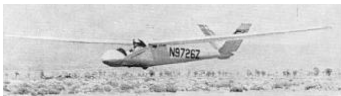
Prue Standard – Owner: William L. Stowers, Lynwood, CA. Built 1961, one of three, 446 lbs. empty, 35:1 g/r
