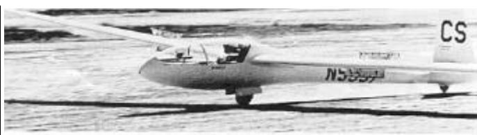
Cirrus – Owners: Tony Terrigno, John Helton, Herb Devies, Bob Embleton. All fiberglass, 753 lbs. Empty. Incl. water ballast, 44:1
