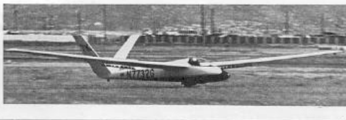
Schempp-Hirth Austria SHK – Owner: Danny Pierson, Compton CA. Built in Germany 1965. 573 lbs. Empty. 39:1 glide ratio
